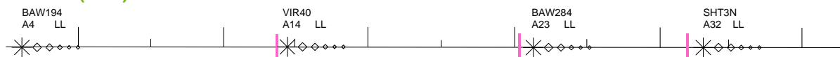
Figure 20: Illustration of Separation Indicator Visualisation of the TBS Distance behind each Lead Aircraft
