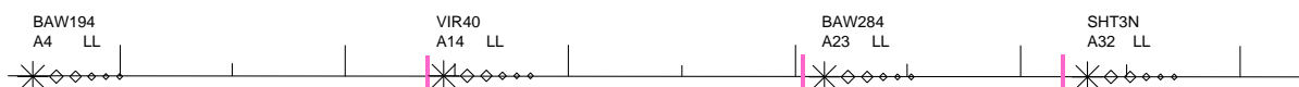
Figure 5: Illustration of Separation Indicator Visualisation of the TBS Distance behind each Lead Aircraft
